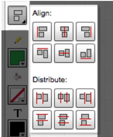
Align moves the shapes into alignment, as pictured by the red line on each button. Distribute spaces shapes out, using the side of the shape highlighted by the red line.
